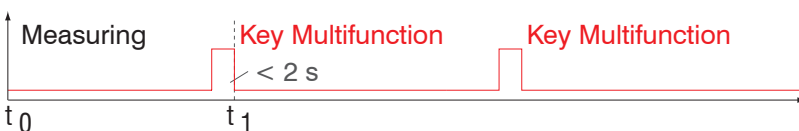
Fig. 63 Flow chart for zeroing, mastering (key Multifunction)
