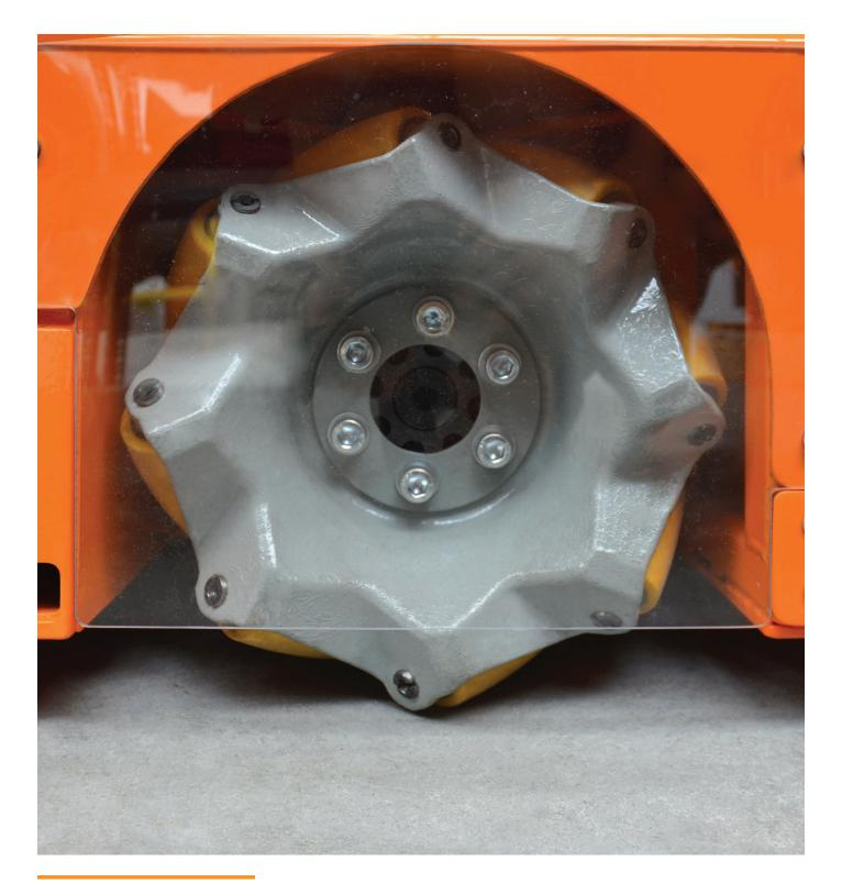
MOBOT® AGV MW mobile self-driving robots are equipped with Mecanum wheels, ensuring the robot's holonomic, i.e. the ability to change the orientation of movement in place. Mecanum wheels consist of freely rotating rollers located at an angle of 45 ° on the circumference of the wheel.
