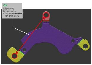
3D measurement of high precision mechanical parts: distance between the holes, planarity and coplanarity of mounting surfaces
