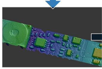
Detailed 3D display due to extremely high z-axis resolution
