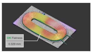
Flatness test of the winding on charging coils
