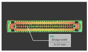
Completeness check of the bridges of a smartphone charging connector plug
