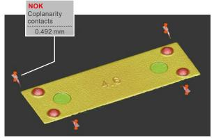
Coplanarity measurement of contacts on electrical components
