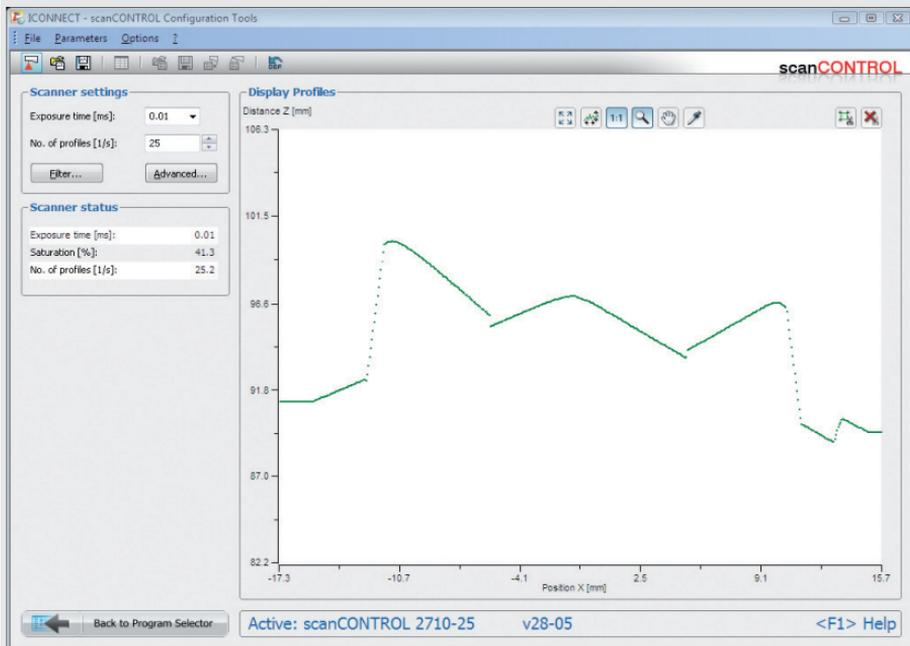
On the left side you can adjust the settings for your measurement task, the right side shows the profile data and information about the measurement.
