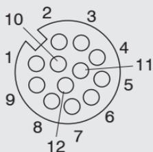
12-pin screw connector, view on solder pin side
