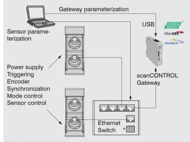
The scanCONTROL Gateway can connect up to four scanCONTROL SMART sensors to the fieldbus. The transmission rate of measurement values is up to 500 Hz. Please refer to the TechNote T026 (scanCONTROL fieldbus integration) for more details.
