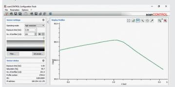
On the left side you can adjust the settings for your measurement task, the right side shows the profile data and information about the measurement.
