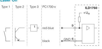
If pin 9 is not connected with pin 6, the laser is off.
