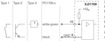
24 V logic (HTL): Low level  $\leq$  3 V; High level ≥ 8 V (max 30 V) 5 V logic (TTL): Low level  $\leq$  0.8 V; High level ≥ 2 V internal pull-up resistor, an open input is detected as High.
