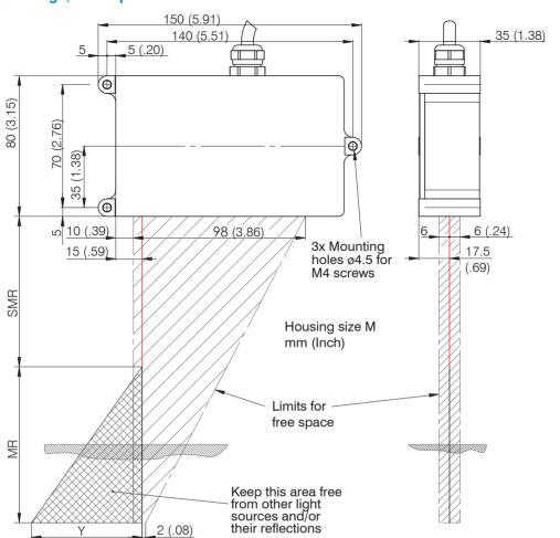
Mount the sensor only to the existing holes on a flat surface. Clamps of any kind are not permitted. Do not exceed torques. The laser beam must be directed perpendicularly onto the surface of the target. In case of misalignment it is possible that the measurement results will not always be accurate.
