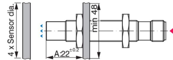
Fig. 5 Assembly, dimensions in mm (not to scale)
