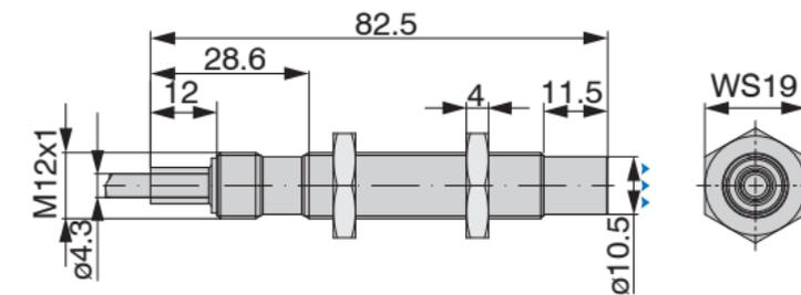
Fig. 3 DT3001-Cx, dimensions in mm (not to scale)
