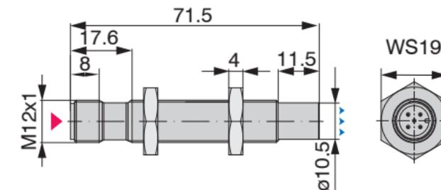
Fig. 2 DT3001-SA, dimensions in mm (not to scale)
