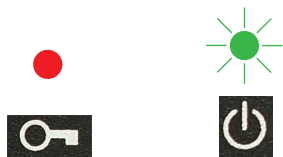
Fig. 21 Green LED flashing, red LED illuminated continuously
